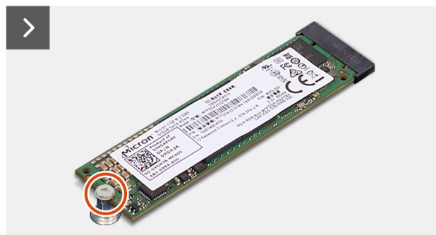
Figure 14. Removing the M.2 2280 solid state drive
