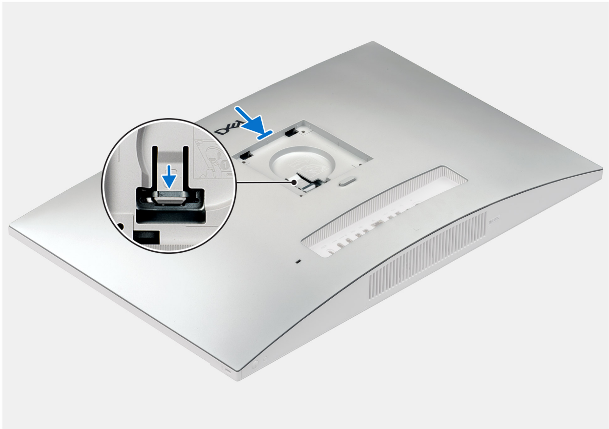
Figure 7. Installing the back cover
