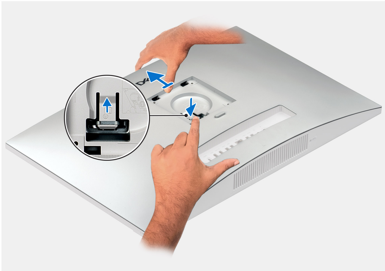
Figure 6. Removing back cover
